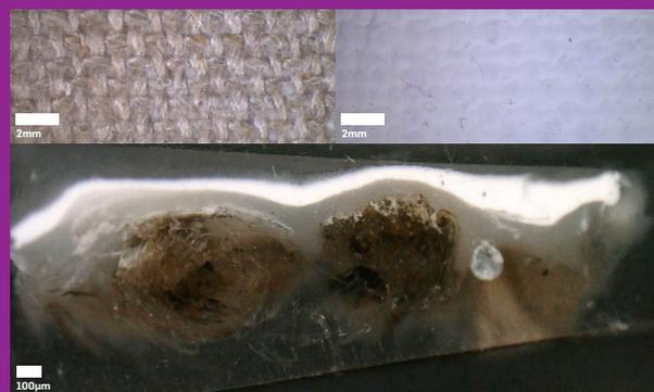
**Figure 6.** Sample QAG 26 — Caravaggio. Top left: reverse showing linen plain weave (11 x 12 threads/cm). Top right: front showing priming surface, micro-cracks noted in priming. Bottom: cross section showing canvas and two priming layers: top layer — acrylic (EA/EHA/EMA/MMA) with titanium white (no chalk), thickness 41.30 µm; bottom layer — styrenated acrylic (EA/MMA) with kaolinite, thickness 86.90µm.
